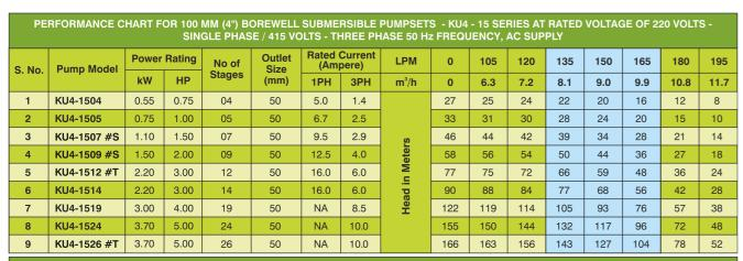
PERFORMANCE CHART FOR 100 MM (4") BOREWELL SUBMERSIBLE PUMPSETS - KU4 -25 SERIES AT RATED VOLTAGE OF 220 VOLTS - SINGLE PHASE / 415 VOLTS - THREE PHASE 50 Hz FREQUENCY. AC SUPPLY
