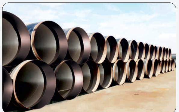
Internal coated pipes at Refinery
