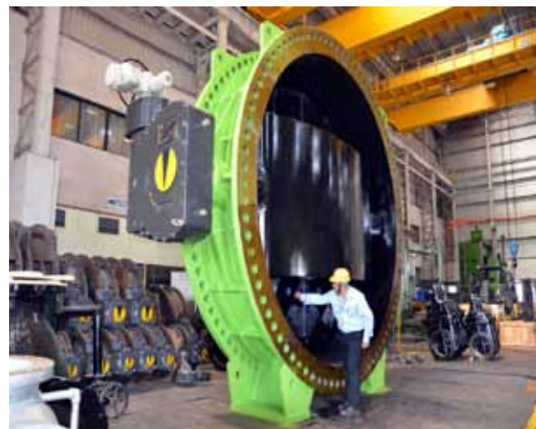
KBL's largest 3800 mm Butterfly Valve manufactured at Kondhapuri Factory
