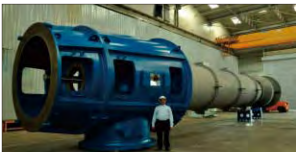
Largest Vertical Turbine pump for sea water intake package of 2 x 520 MW Vizag Power Project of Hinduja National Corporation Limited (HNPC).
