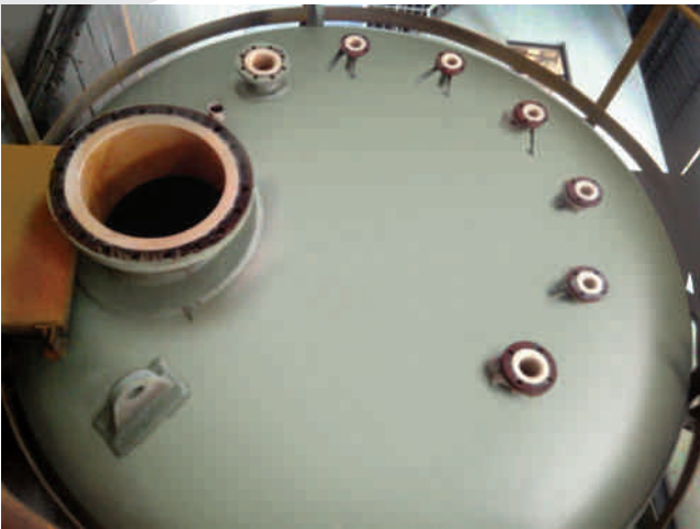
Internal chemical resistant lining done for Chemical storage tank
