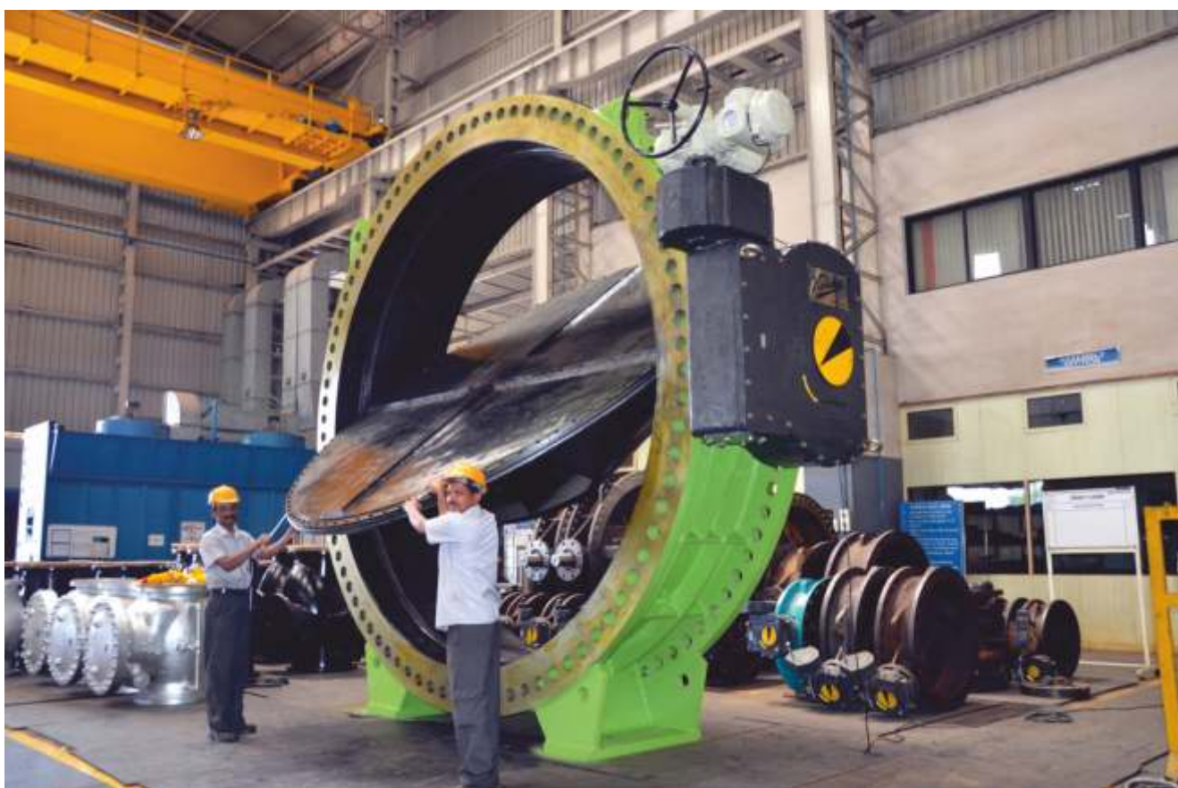
Assembly of 3800 mm Motorized Butterfly Valve
