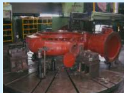
FRANCIS SPIRAL CASING MACHINING ON SK40 VTL
