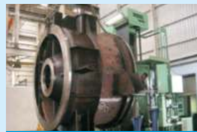
TUBULAR KAPLAN CASING MACHINING ON WOTON CNCHBM
