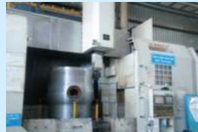
KAPLAN RUNNER HUB MACHINING ON CNC VBM
