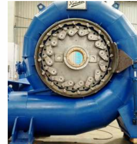
FRANCIS TURBINE AT WORKS
