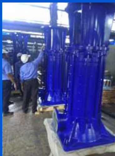
RKB 200/37 – 7-Stage Pump in Vertical Execution installed on-site
