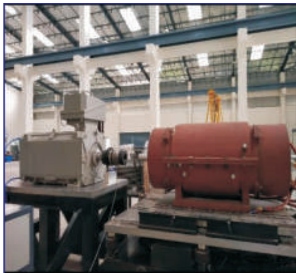
MEA make 350 KW Motor Test Bed for Urja Project
