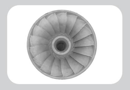
Francis Runner Casting Manufactured With 3D Print Core (Weight: 2.2 MT)
