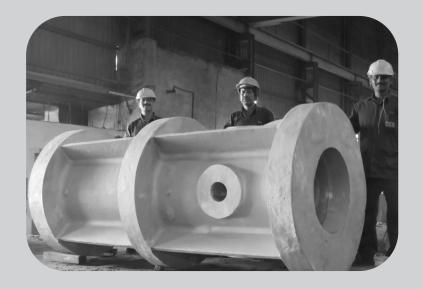
Largest Stainless Steel Casting Produced (Weight: 8.8 MT)
