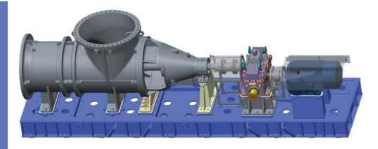
KBL recently developed a large Vertical Turbine pumpset. It is a single-stage Horizontal Axial Flow Pump developed for use in the Circulation of Fermentation Broth. The pump has a discharge capacity up to 12960 m3/hr at 365 rpm and 10368 m3/hr at 285 rpm. The castings, shafting, sleeves, and
