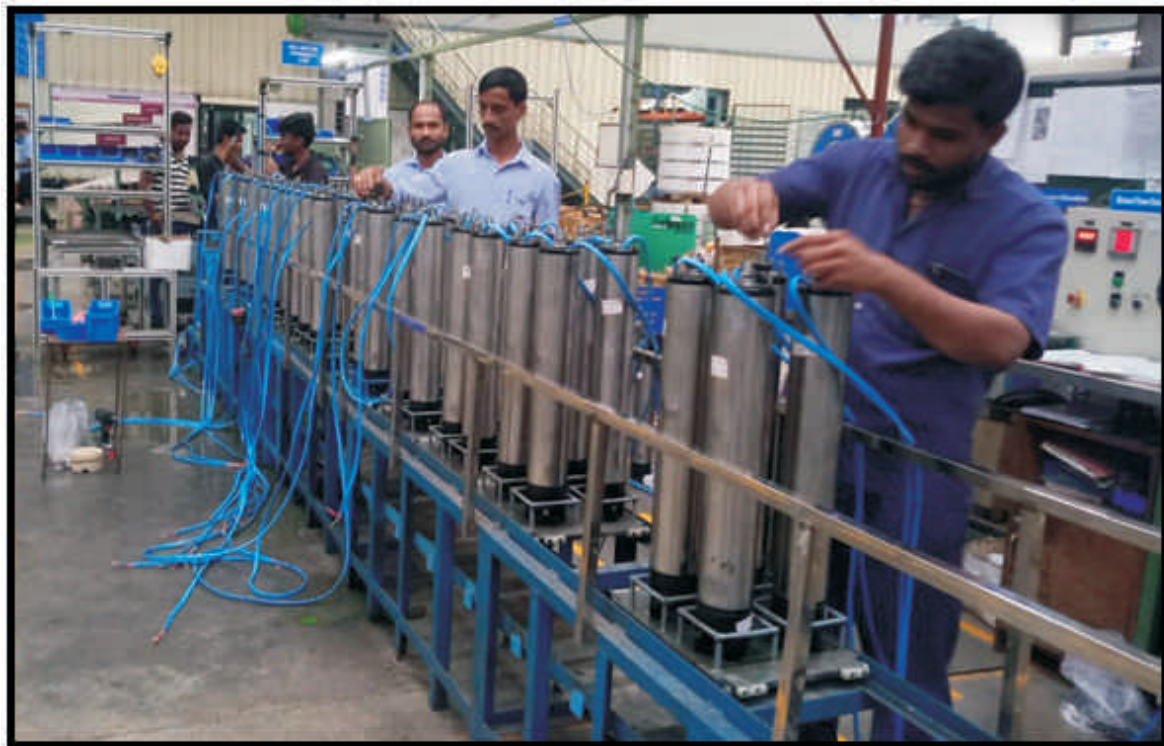
Installed Conveyor for Water Filled Submersible Motor Assembly
