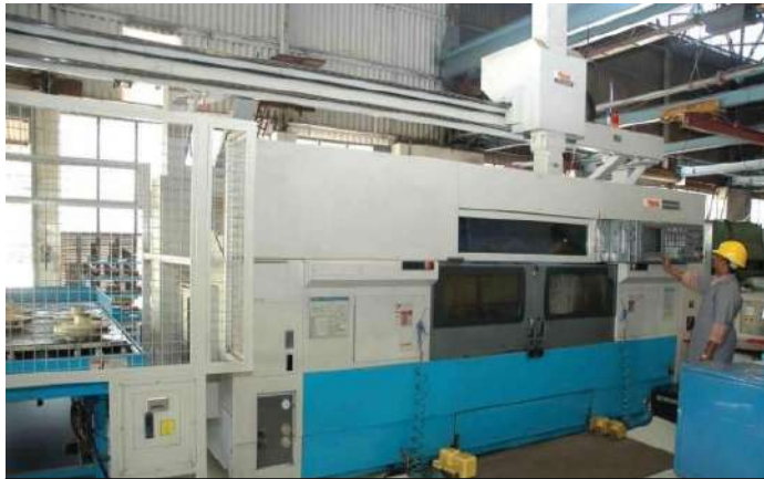
Fully automatic twin spindle, twin turret machine
