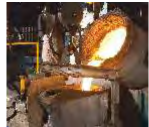
A large pump casting being poured.
