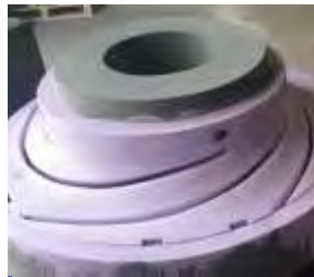
An impeller core of a large pump is being set in the mould (3D printed).
