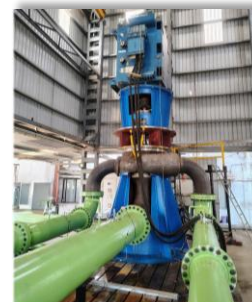
Primary Cooling Pump (PCP) for Pressurized Heavy Water Reactor (PHWR)
